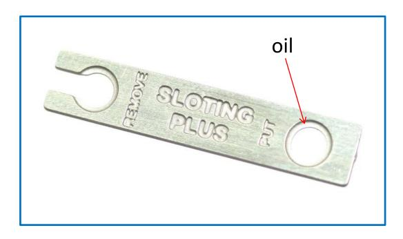
Put a drop of oil as indicated in the photo and the washer will adhere, it will not fall and you will work comfortably.
