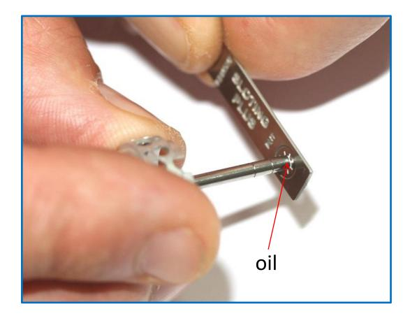
Put a drop of oil on the end of the semi-axle to facilitate the insertion of the toothed washer.
