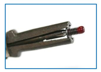
Put screw fixer or nail polish on the threaded end of the screw as shown in the picture. Remember to put little amount.
