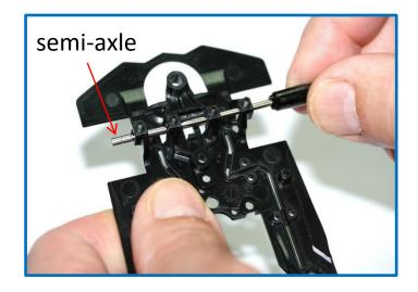
With a single semi-axle, and once the screw is placed in the thread, it will be very easy to screw on the assembly and you will be able to tighten or loose harder. With the other semi-axle already in place, and the hexagonal screws completely unscrewed, insert the Phillips screwdriver as it's show in the picture to tighten or loose.
