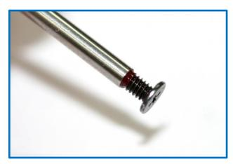
Our recommendation, without detracting from the use of professional screw fixers, is to use nail polish and, if possible, colored to identify it when we are using it.
