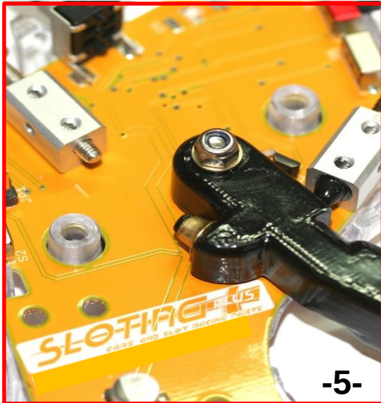
Photo 5: Place the self-locking nut and tighten gently, ensuring the trigger functions correctly. Do not overtighten; tighten only until it stops.
