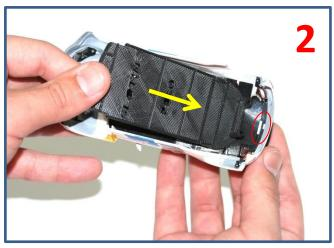
Fit the hole of the base/support in the rear tab of the body (red circle).
