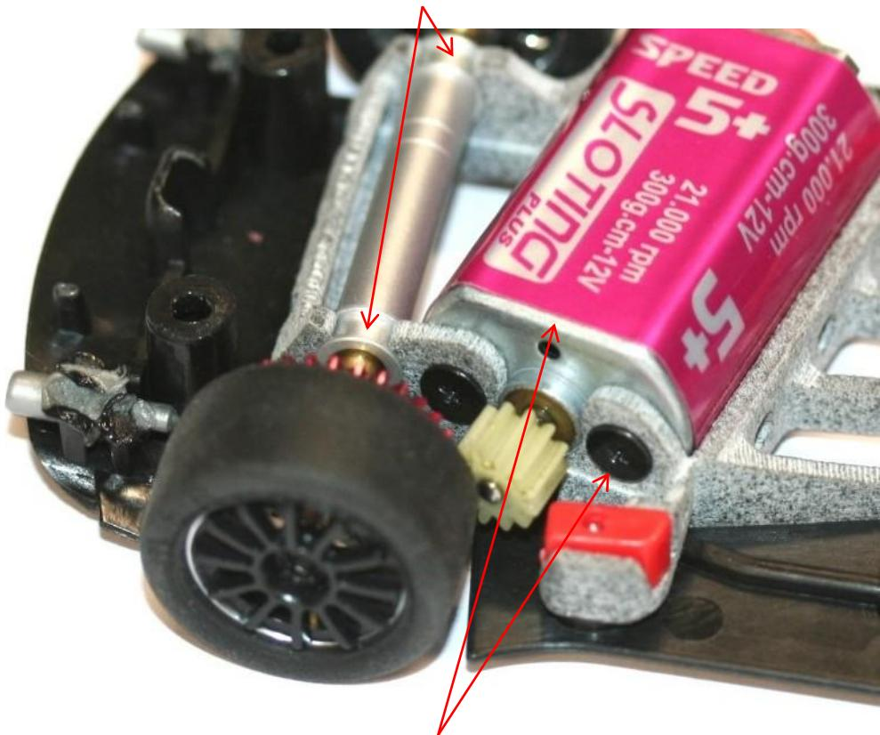
Don't force the motor when inserting it or when tightening the screws that hold it in place.
