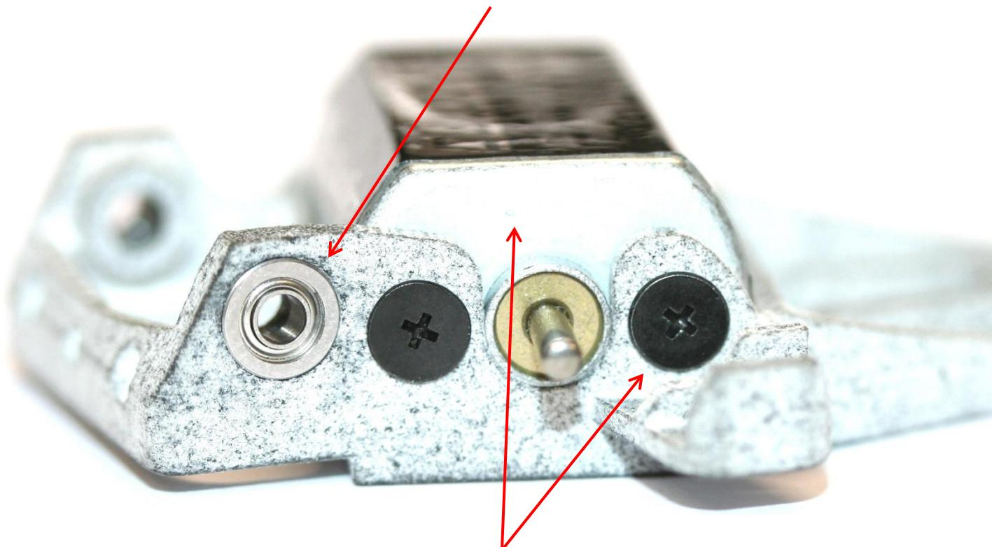
Don't force the motor when inserting it or when tightening the screws that hold it in place.
