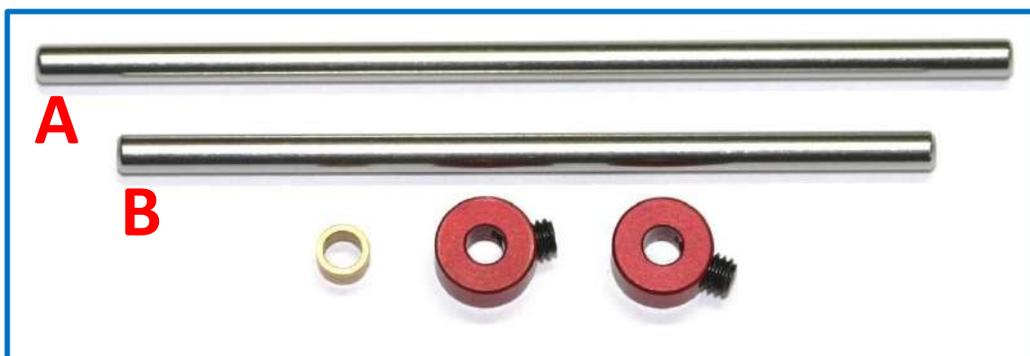
We will use an Alfa Romeo DTM model from the Slot.it as example and using two  $\varnothing 15.9$  mm BBS rims. x 8.5mm wide -with their respective Allen grubs-, a set of grip -0- tyres, two 2 mm brass spacers long and two standard 0.10 mm steel spacers of thickness.
