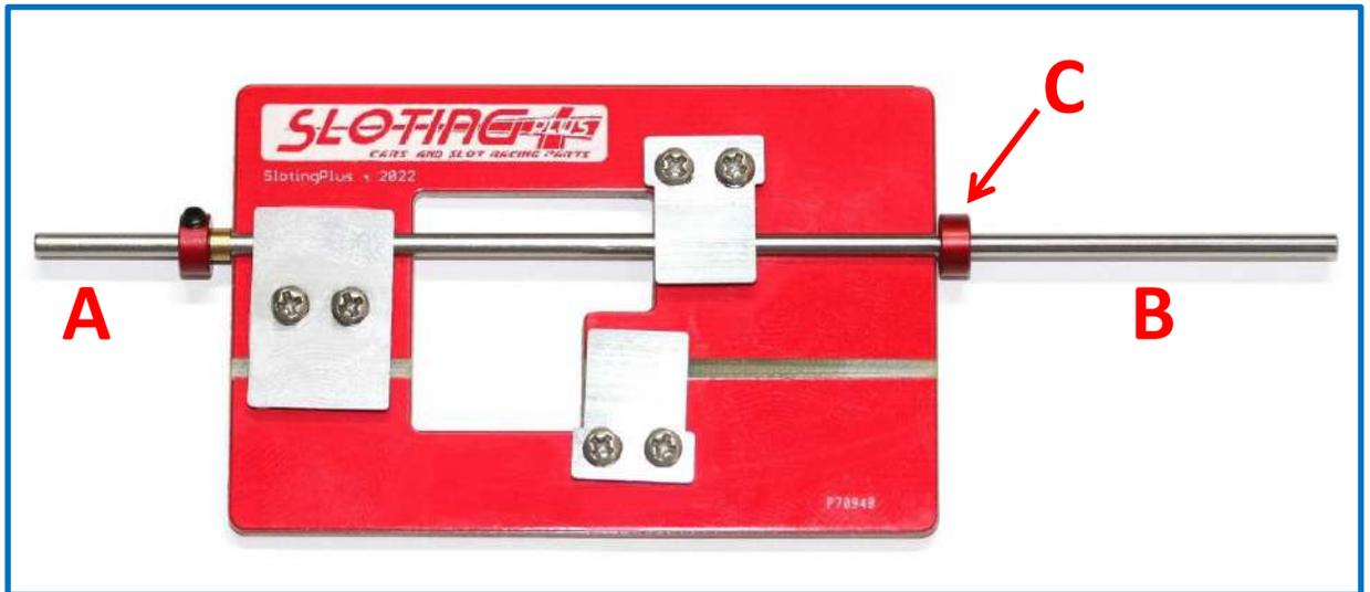
Now place the two semi-axes, taking special care that the marks are facing each other (lower image) and also place the small guide axle inside.
