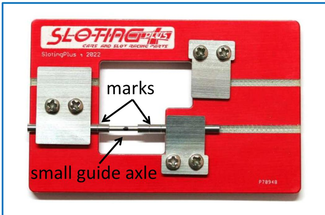
Take special care to level the left semi-axle with the red base as indicated in the lower picture.
