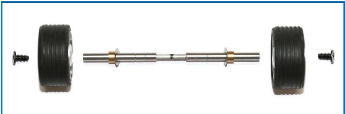
Remember that it will be necessary to use "soft" screw fixer or nail polish to prevent the screws from coming loose.
