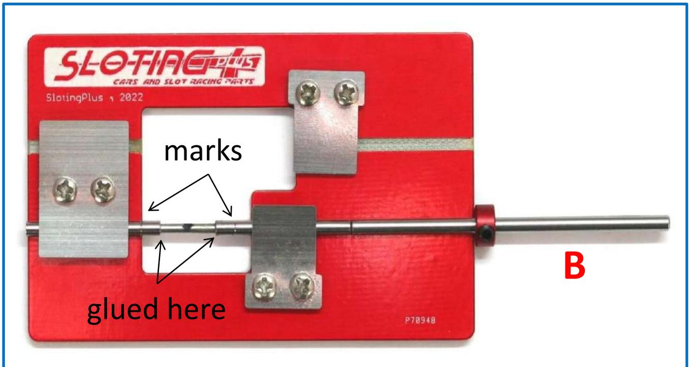
**ATTENTION:** Glue the set with Cyanoclorate type glue but using **-VERY LITTLE AMOUNT-** quantity because the glue will act by capillarity and a very small quantity is sufficient. Help yourself with a toothpick or similar to deposit the glue.
