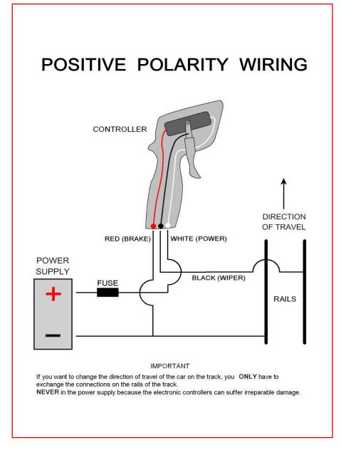
Correct way to connect the EVO PRO controller to the track and to the power supply.
